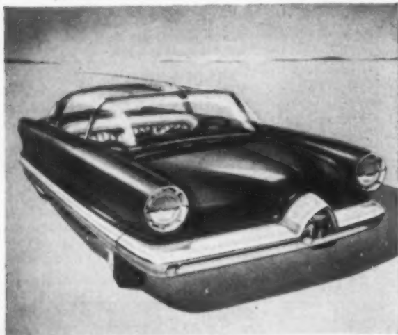
Streamlined hard-top has doors that curve up into roof, making it easier to enter and leave. Note how bumper circles car completely.
